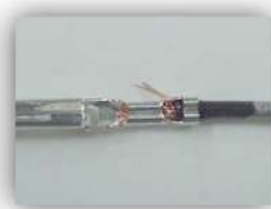
Missing strands of wire
