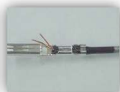
Insulation part in conductor crimp (Wire strands missing)
