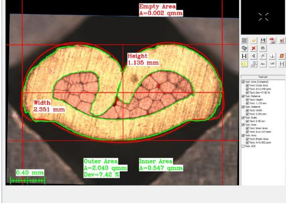
Image monitoring and analyzing can be processed easily. Crimp height, Crimp width, Compound ratio, etc. are measured automatically. World top car makers' templates for report are pre-installed. This is the world standard software.
