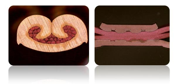
Sample of crimped terminal can be cut, ground and done with electrolyte etching. The finished samples' cut faces are visually monitored and analyzed. All processes are compactly arranged in the compact system. Even the hardened samples and insulation barrel cut samples are available, too.
